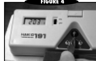
Hakko digital thermometer used to verify wedge temperature.
